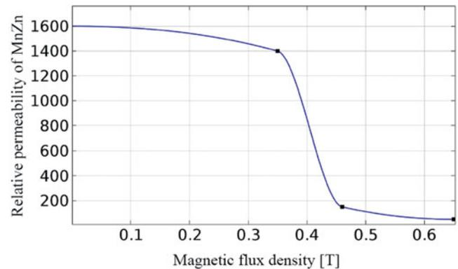
Figure 3. Relative permeability of MnZn core versus magnetic flux density.
