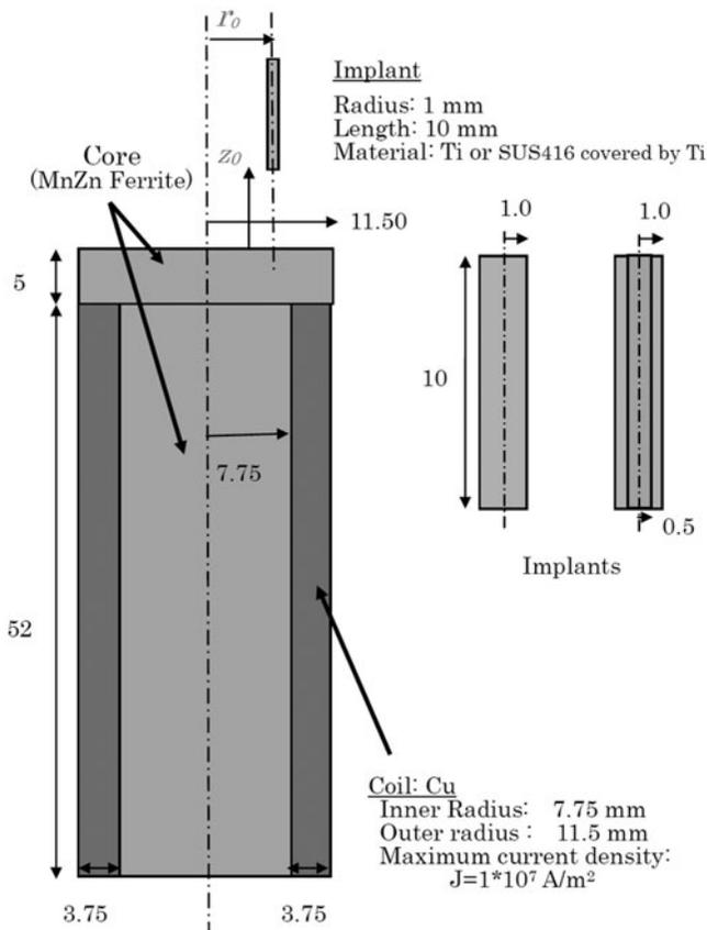
Figure 2. Schematic illustration of the applicator and implants.
