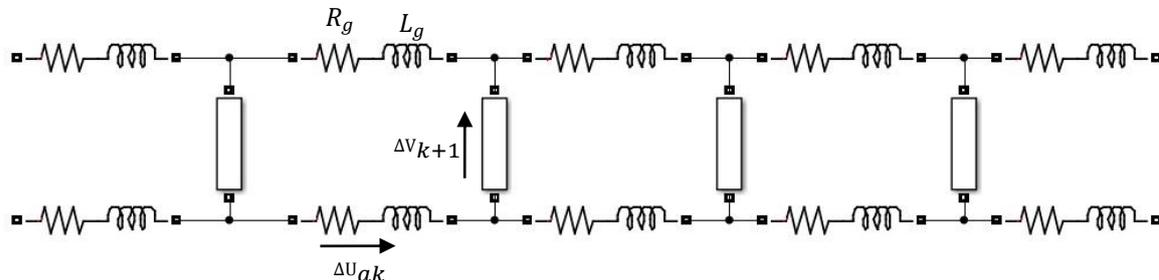
Fig. 1. Short circuit ring of the rotor bars
