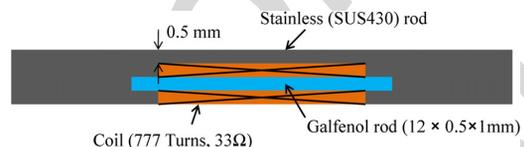
Fig. 1. Structure of the unimorph vibration energy harvester.
