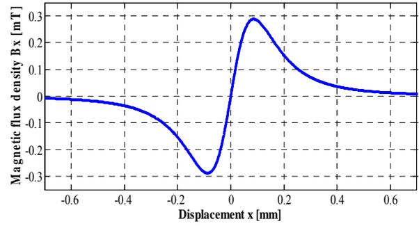
Fig. 4 x-component of magnetic flux density versus distance.
