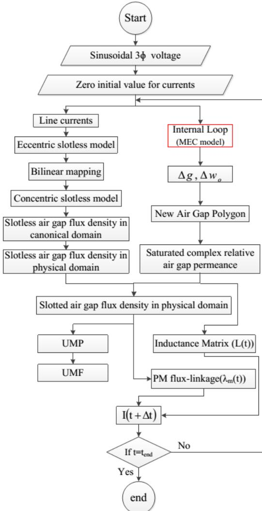
Fig. 1. General flowchart for transient analysis
