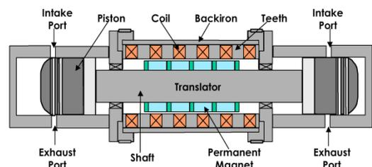
Fig. 1. Free-piston alternator-engine with movable permanent magnet<sup>(1)</sup>
